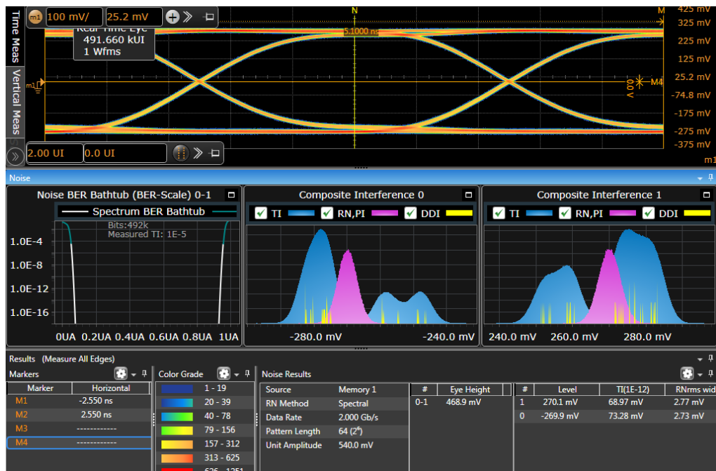
Figure 10. Hardware and visual triggering to capture physical layer anomalies
