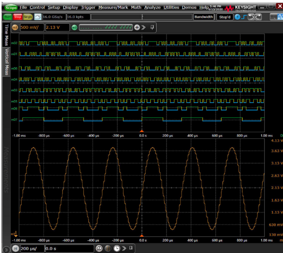
Figure 5. Synchronous analog and digital domain correlation with MSO capabilities
