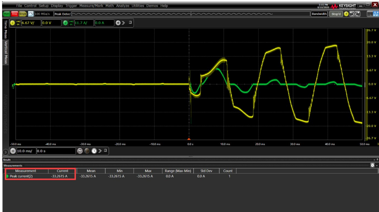
Figure 9. Inrush current measurements. The yellow signal above is the voltage waveform turning on. The green one is the current wave going from zero amps up and then to a steady state.
