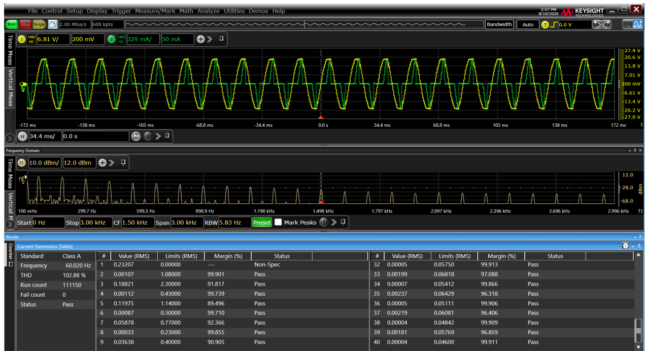
Figure 6. Current harmonics measurements in a tabular format
