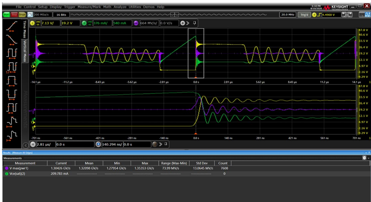
Figure 13. Slew rate measurement of the voltage waveform during the transistor's turn-off phase
