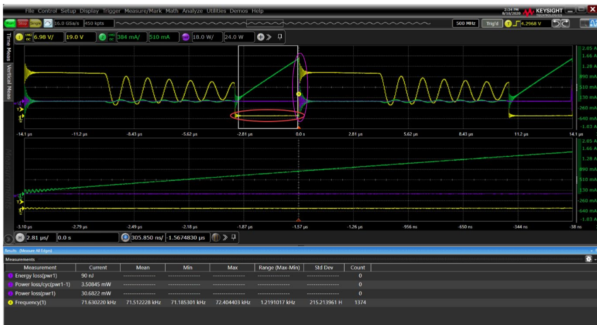
Figure 11. Power and energy losses during the conduction phase. The transistor's saturation voltage level (circled in red) is magnitudes lower than the peak-to-peak voltage (circled in pink at right) during the conduction phase of the switching device (e.g., transistor) in the power supply.
