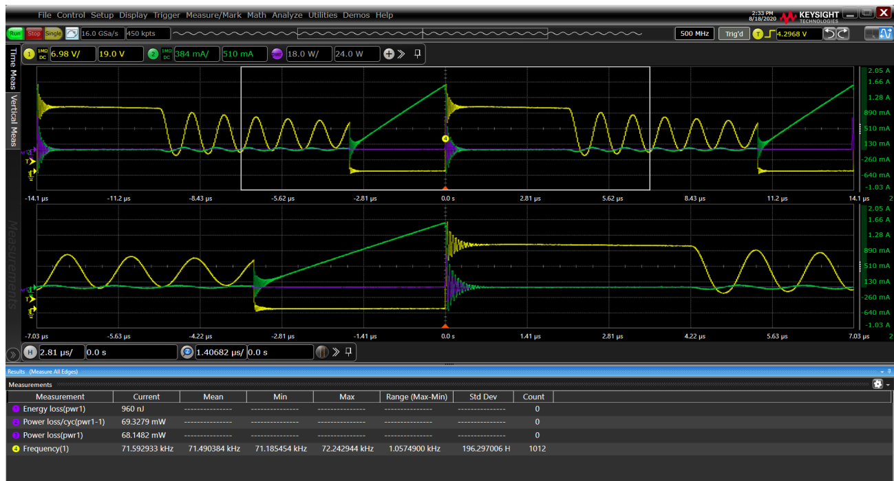
Figure 10. Power and energy losses over one switching cycle
