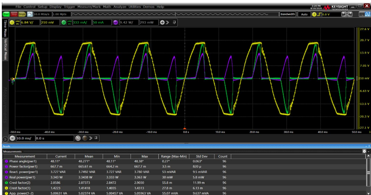
Figure 5. Input power quality measurements. Here, the yellow sinusoidal waveform is voltage, the green pulsed waveform is current, and the purple is the power waveform, which uses the scope's waveform math ( P=V \times I ).
