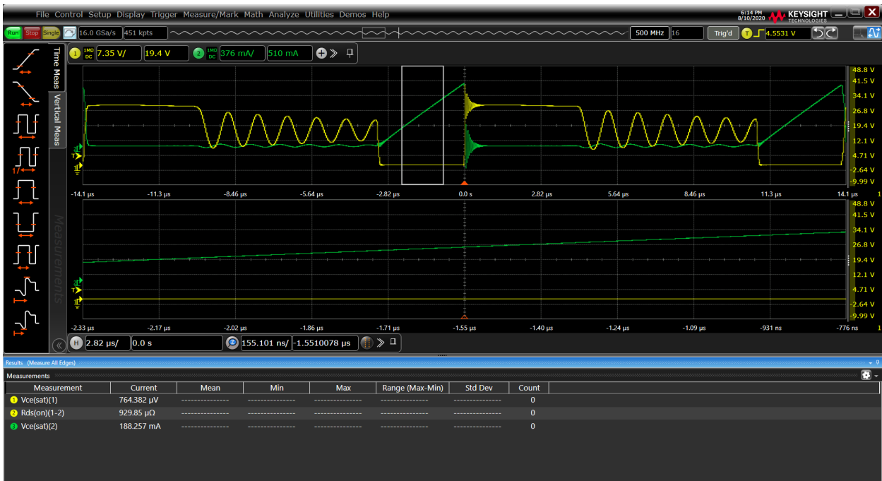
Figure 12. Measuring R_{ds} (on)
