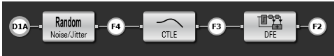
Figure 9. Reference receiver noise and equalizer components
