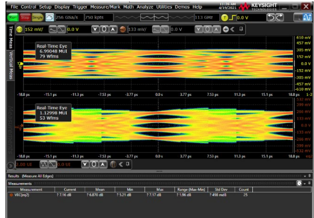
Figure 15. Running a Tx test on the UXR
