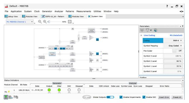
Figure 23. The graphical user interface offers multiple views that can be defined by the user. This example shows the system view on the left side and the pattern generator data output with the PAM4 coding and level linearity parameters at the right.
