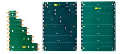
Figure 16. Emulate channel loss for receiver margin testing with Keysight's ISI channel boards
