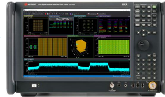
Modulation analysis of each 100 MHz carrier
