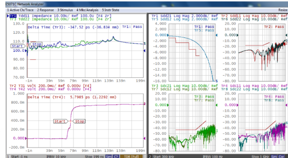
Test Result Example – E5071C screenshot of limit test
