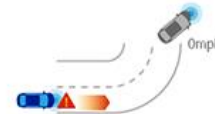
Blind curve/ Local hazard warning
