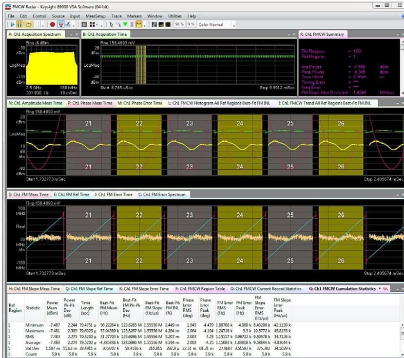
View spectrum and time domain results on multi-chirp FM signals. In the image pictured here highlighting six selected FM regions (number 21 through 26) in synchronized time domain traces. The FMCW cumulative statistic table below provides accumulated results over all detected regions.
