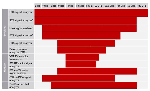
1. Up to 2.2 T Hz with external mixing
