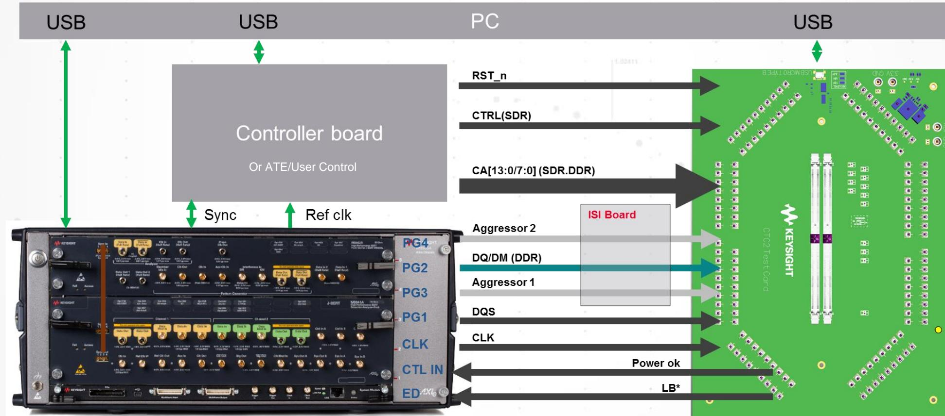
\* There can be one or two loopback signals depending on the device under test
