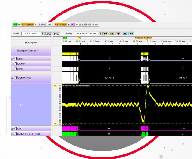
**Correlate memory analysis to Power Integrity or signal integrity probing**
