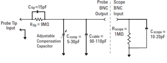
Where  $C_{parallel} = C_{comp} + C_{cable} + C_{scope}$
