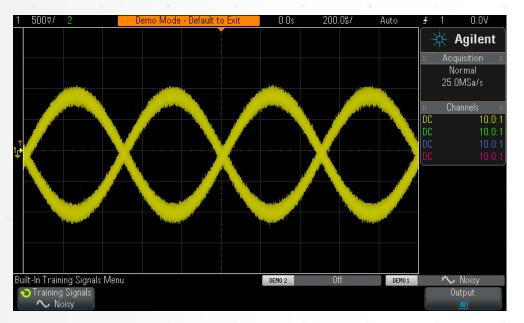
Rising edge trigger – Scope triggers on high frequency noise during a falling edge of sine wave 🙁 Rising edge trigger, HF Reject – Scope correctly triggers on high frequency noise
