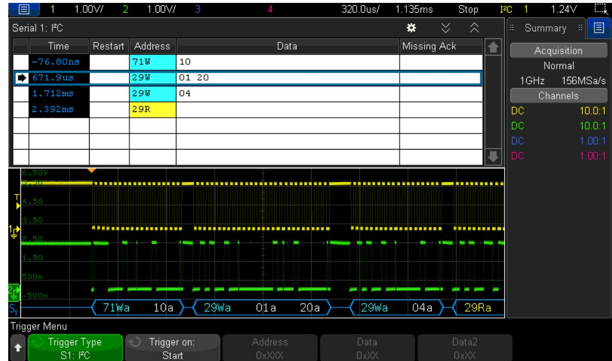
Example: Triggering on an I<sup>2</sup>C serial bus
