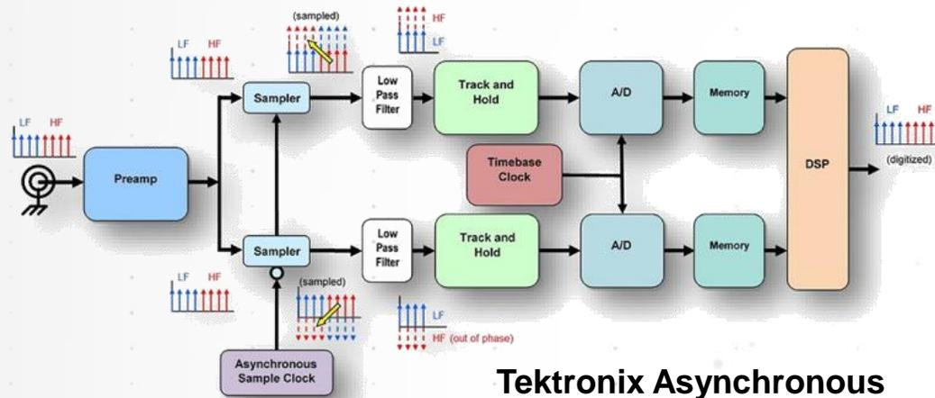
**Tektronix Asynchronous Time Interleave (ATI)**
