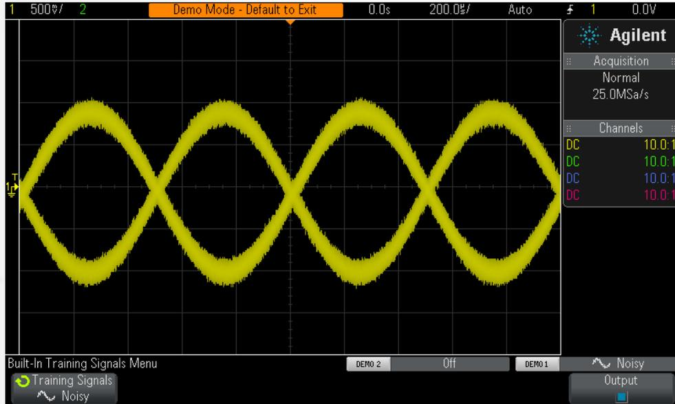
Rising edge trigger – Scope triggers on high frequency noise during a falling edge of sine wave ☹️
