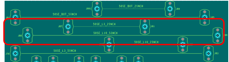
Single-End transmission line
